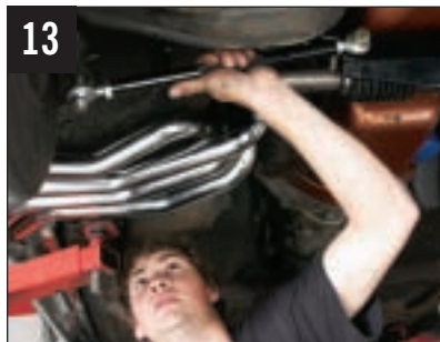
13 Adjustments to the toe-in can be made by simply turning the tie rod, as the tie rod ends are both left and right hand threaded. Once everything was in place, the jam nuts were tightened on the rod ends.
