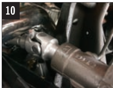
10 We also encountered clearance issues with the universal joint and the factory side pipe headers. Some adjustments were made to the primary tube using a prybar to gain clearance.
