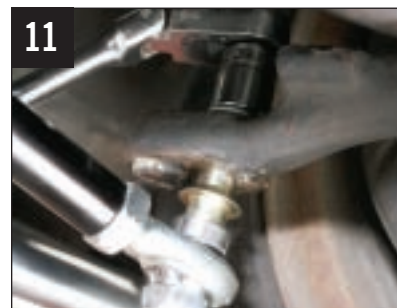
11 A set of tapered seat adapters is provided with the kit. These allow the tie rod ends to be connected safely to the spindles.
