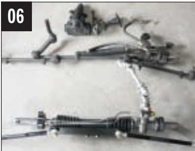
06 The differences between the OEM steering system and the new rack system become apparent once they're laid beside each other. It's easy to see why the new system is 15 pounds lighter.
