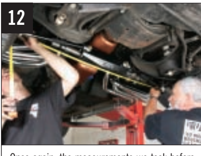
12 Once again, the measurements we took before disassembly came in handy. The camber and caster were not altered during this conversion, although you'll want to send it to the alignment shop before racking up too many miles.
